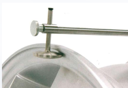
Checking plane parallelism to the inner rim flange
